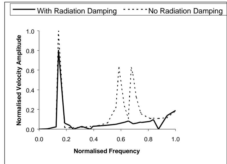
Fig. 1: Effect of radiation damping on vibration amplitude.
