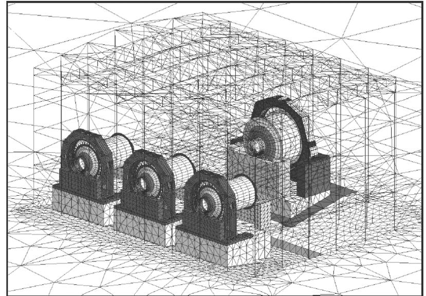
**Fig. 5: Model of a complete grinding facility.**
