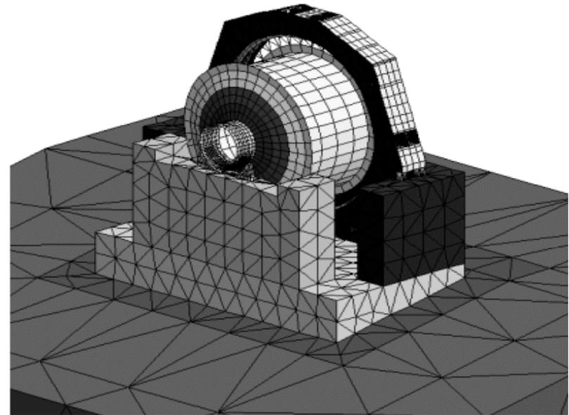
Fig. 3: Part model of the SAG mill system.
