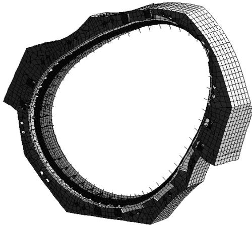
Fig. 2: Dominant mode of stator vibration (SAG Mill).
